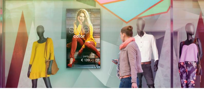
Please be aware light spots in a shopping window pointed at a display can also cause heating up of the panel, so investigate the environment very closely to prevent heating up the display. Also sunlight-reflection from another reflecting surface (e.g. a different window) can cause local "heat pockets" and might cause damage to the display.
